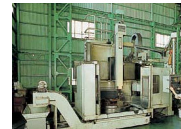
NC立旋盤 (東芝機械製・ATC付) NC VERTICAL LATHE (TOSHIBA MACHINE'S, ATC CONTROLLED)
